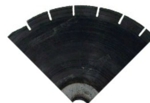
Blade Will Not Cut: Blade is glazed or too hard for the job
